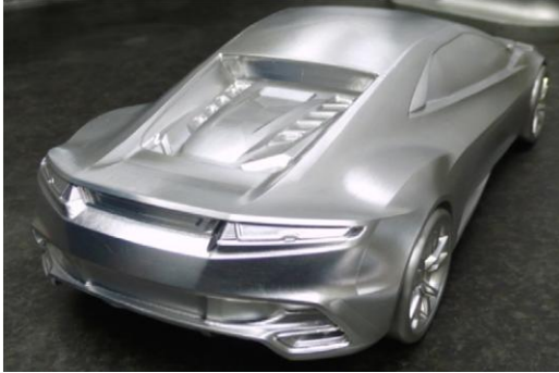
Model Car – Solid Aluminium, Machined Finish
