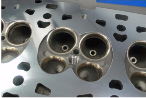
Cylinder Head – Machined from Casting
