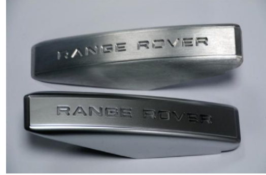
Side Fins – Machined and Hand Finished
