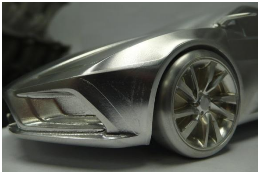
Model Car – Solid Aluminium, Machined Finish
