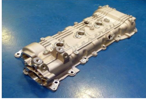
Cam Cover – Machined from Aluminium Casting
