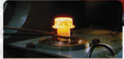
Closed Die Upset Forging
