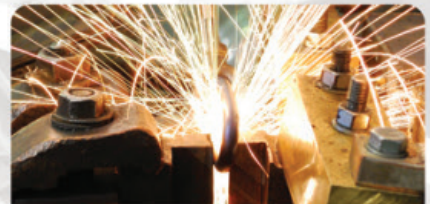
Flash Butt Welding
